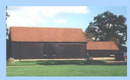
Figure 100: A barn conversion in the borough, showing the general approach of no windows on the public side to maintain the agricultural appearance, including no rooflights, dormers or chimneystacks.
